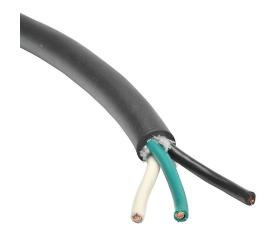
Southwire portable cord, unshielded, SEOOW, 600V, 3 conductors (includes ground), 16 AWG, TPE conductor insulation material, black, white and green, TPE jacket, black, cut to length.
