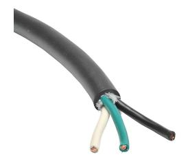
Southwire portable cord, unshielded, SEOOW, 600V, 3 conductors (includes ground), 14 AWG, TPE conductor insulation material, black, white and green, TPE jacket, black, cut to length.
