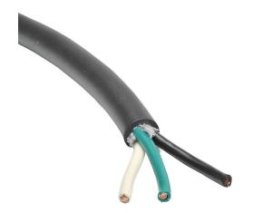
Southwire portable cord, unshielded, SEOOW, 600V, 3 conductors (includes ground), 12 AWG, TPE conductor insulation material, black, white and green, TPE jacket, black, cut to length.
