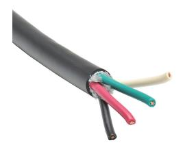
Southwire portable cord, unshielded, SEOOW, 600V, 4 conductors (includes ground), 10 AWG, TPE conductor insulation material, black, white, red and green, TPE jacket, black, cut to length.
