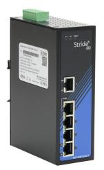
STRIDE industrial unmanaged PoE+ switch, IEEE 802.3af/at, 120W, 5 ports, (4) PoE+ 10/100Base-T (RJ45) and (1) Ethernet 10/100Base-T (RJ45) port(s), 12-36 VDC nominal input, -40 to +75 deg C, NEMA TS2, 35mm DIN rail or panel mount, hazardous location rated.
