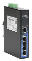
STRIDE industrial unmanaged PoE+ switch, IEEE 802.3af/at, 120W, 5 ports, (4) PoE+ 10/100Base-T (RJ45) and (1) Ethernet 10/100Base-T (RJ45) port(s), 48-55 VDC nominal input, -40 to +75 deg C, 35mm DIN rail or panel mount, hazardous location rated.
