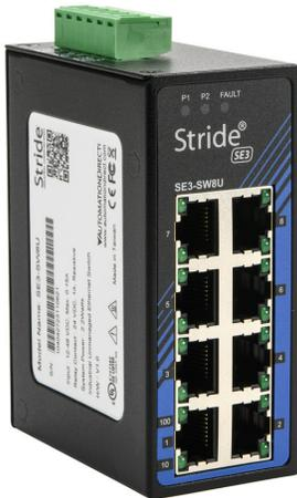
STRIDE industrial unmanaged Ethernet switch, 8 ports, (8) Ethernet 10/100Base-T (RJ45) port(s), -10 to +65 deg C, metal housing, IP30, 35mm DIN rail or panel mount.
