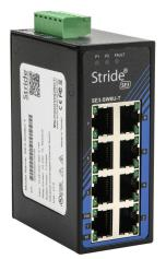
STRIDE industrial unmanaged Ethernet switch, 8 ports, (8) Ethernet 10/100Base-T (RJ45) port(s), -40 to +75 deg C, metal housing, IP30, 35mm DIN rail or panel mount.
