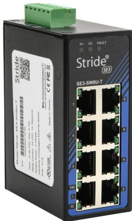
STRIDE industrial unmanaged Ethernet switch, 8 ports, (8) Ethernet 10/100Base-T (RJ45) port(s), -40 to +75 deg C, metal housing, IP30, 35mm DIN rail or panel mount.
