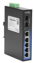
STRIDE industrial unmanaged Ethernet switch, 7 ports, (5) Ethernet 10/100Base-T (RJ45) and (2) SFP combo Gigabit port(s), -40 to +75 deg C, metal housing, IP30, 35mm DIN rail or panel mount.
