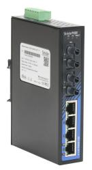
STRIDE industrial unmanaged Ethernet switch, 6 ports, (4) Ethernet 10/100Base-T (RJ45) and (2) multi-mode ST 100FX fiber port(s), -40 to +75 deg C, metal housing, IP30, 35mm DIN rail or panel mount.
