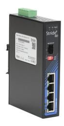
STRIDE industrial unmanaged Ethernet switch, 5 ports, (4) Ethernet Gigabit (RJ45) and (1) SFP combo Gigabit port(s), -40 to +75 deg C, metal housing, IP30, 35mm DIN rail or panel mount.
