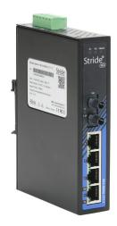
STRIDE industrial unmanaged Ethernet switch, 5 ports, (4) Ethernet 10/100Base-T (RJ45) and (1) multi-mode ST 100FX fiber port(s), -40 to +75 deg C, metal housing, IP30, NEMA TS2, 35mm DIN rail or panel mount.
