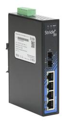
STRIDE industrial unmanaged Ethernet switch, 5 ports, (4) Ethernet 10/100Base-T (RJ45) and (1) multi-mode SC 100FX fiber port(s), -40 to +75 deg C, metal housing, IP30, NEMA TS2, 35mm DIN rail or panel mount.
