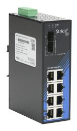
STRIDE industrial unmanaged Ethernet switch, 10 ports, (8) Ethernet Gigabit (RJ45) and (2) SFP combo Gigabit port(s), -40 to +75 deg C, metal housing, IP30, 35mm DIN rail or panel mount.
