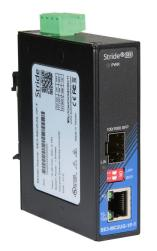
STRIDE industrial unmanaged Ethernet media converter, 2 ports, (1) Ethernet 10/100/1000Base-T (RJ45) and (1) SFP combo Gigabit port(s), -40 to +80 deg C, metal housing, IP30, 35mm DIN rail or panel mount.
