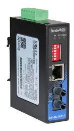
STRIDE industrial unmanaged Ethernet media converter, 2 ports, (1) Ethernet 10/100Base-T (RJ45) and (1) multi-mode ST 100FX fiber port(s), (1) Form A (SPST) relay, -40 to +80 deg C, metal housing, IP30, 35mm DIN rail or panel mount.
