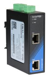
STRIDE industrial unmanaged, PoE++ injector, IEEE 802.3af/at/bt, up to 90W, 2 ports, (1) PoE++ Gigabit (RJ45) and (1) Ethernet Gigabit (RJ45) port(s), 9-55 VDC nominal input, -40 to +75 deg C, 35mm DIN rail or panel mount.
