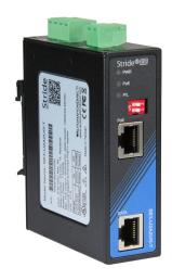
STRIDE industrial unmanaged, PoE++ injector, IEEE 802.3af/at/bt, up to 100W, 2 ports, (1) PoE++ Gigabit (RJ45) and (1) Ethernet Gigabit (RJ45) port(s), 9-55 VDC nominal input, -40 to +75 deg C, 35mm DIN rail or panel mount.
