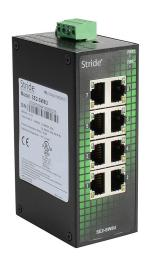
STRIDE industrial unmanaged Ethernet switch, 8 ports, (8) Ethernet 10/100Base-T (RJ45) port(s), -10 to +60 deg C, metal housing, IP30, 35mm DIN rail mount.
