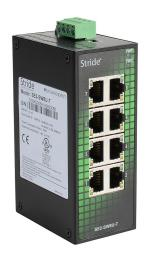
STRIDE industrial unmanaged Ethernet switch, 8 ports, (8) Ethernet 10/100Base-T (RJ45) port(s), -40 to +75 deg C, metal housing, IP30, 35mm DIN rail mount.
