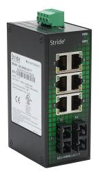
STRIDE industrial unmanaged Ethernet switch, 8 ports, (6) Ethernet 10/100Base-T (RJ45) and (2) multi-mode SC 100FX fiber port(s), -40 to +75 deg C, metal housing, IP30, 35mm DIN rail mount.
