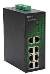
STRIDE industrial managed Ethernet switch, 8 ports, (8) Ethernet 10/100Base-T (RJ45) port(s), EtherNet/IP and Modbus TCP, -40 to +75 deg C, metal housing, IP40, 35mm DIN rail mount.
