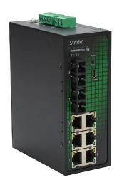
STRIDE industrial managed Ethernet switch, 8 ports, (6) Ethernet 10/100Base-T (RJ45) and (2) multi-mode SC 100FX fiber port(s), EtherNet/IP and Modbus TCP, -40 to +75 deg C, metal housing, IP40, 35mm DIN rail mount.
