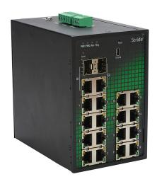
STRIDE industrial managed Ethernet switch, 18 ports, (16) Ethernet 10/100Base-T (RJ45), (2) Ethernet combo Gigabit (RJ45) and (2) SFP combo Gigabit port(s), EtherNet/IP and Modbus TCP, -40 to +75 deg C, metal housing, IP40, 35mm DIN rail mount.
