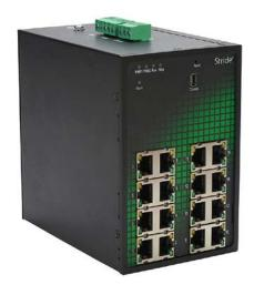
STRIDE industrial managed Ethernet switch, 16 ports, (16) Ethernet 10/100Base-T (RJ45) port(s), EtherNet/IP and Modbus TCP, -40 to +75 deg C, metal housing, IP40, 35mm DIN rail mount.
