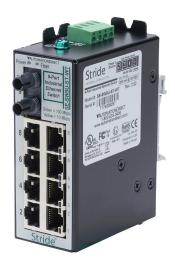
STRIDE industrial unmanaged Ethernet switch, 9 ports, (8) Ethernet 10/100Base-T (RJ45) and (1) multi-mode ST 100FX fiber port(s), -40 to +85 deg C, metal housing, IP40, 35mm DIN rail mount.
