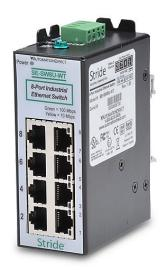
STRIDE industrial unmanaged Ethernet switch, 8 ports, (8) Ethernet 10/100Base-T (RJ45) port(s), -40 to +85 deg C, metal housing, IP40, 35mm DIN rail mount.
