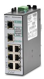
STRIDE industrial managed Ethernet switch, 8 ports, (8) Ethernet 10/100Base-T (RJ45) port(s), Modbus TCP, -40 to +75 deg C, metal housing, IP40, 35mm DIN rail mount.
