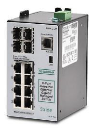
STRIDE industrial managed Ethernet switch, 8 ports, (8) Ethernet Gigabit (RJ45) and (4) SFP combo Gigabit port(s), Modbus TCP, -40 to +75 deg C, metal housing, IP40, 35mm DIN rail mount.
