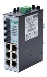
STRIDE industrial managed Ethernet switch, 8 ports, (6) Ethernet 10/100Base-T (RJ45) and (2) multi-mode ST 100FX fiber port(s), Modbus TCP, -40 to +75 deg C, metal housing, IP40, 35mm DIN rail mount.
