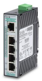
STRIDE industrial unmanaged Ethernet switch, 5 ports, (5) Ethernet 10/100Base-T (RJ45) port(s), -10 to +60 deg C, plastic housing, IP40, 35mm DIN rail mount.
