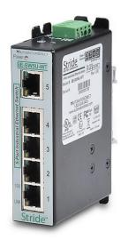
STRIDE industrial unmanaged Ethernet switch, 5 ports, (5) Ethernet 10/100Base-T (RJ45) port(s), -40 to +85 deg C, metal housing, IP40, 35mm DIN rail mount.
