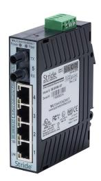
STRIDE industrial unmanaged Ethernet switch, 5 ports, (4) Ethernet 10/100Base-T (RJ45) and (1) multi-mode ST 100FX fiber port(s), -10 to +60 deg C, plastic housing, IP40, 35mm DIN rail mount.
