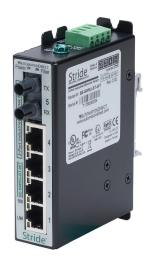
STRIDE industrial unmanaged Ethernet switch, 5 ports, (4) Ethernet 10/100Base-T (RJ45) and (1) multi-mode ST 100FX fiber port(s), -40 to +85 deg C, metal housing, IP40, 35mm DIN rail mount.
