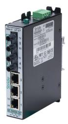
STRIDE industrial managed Ethernet switch, 5 ports, (3) Ethernet 10/100Base-T (RJ45) and (2) multi-mode ST 100FX fiber port(s), Modbus TCP, -40 to +75 deg C, metal housing, IP40, 35mm DIN rail mount.
