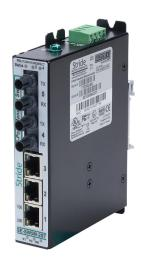
STRIDE industrial managed Ethernet switch, 5 ports, (3) Ethernet 10/100Base-T (RJ45) and (2) multi-mode ST 100FX fiber port(s), Modbus TCP, -40 to +75 deg C, metal housing, IP40, 35mm DIN rail mount.
