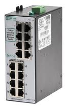
STRIDE industrial managed Ethernet switch, 16 ports, (16) Ethernet 10/100Base-T (RJ45) port(s), Modbus TCP, -40 to +75 deg C, metal housing, IP40, 35mm DIN rail mount.
