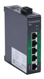
StrideLinx Pro industrial VPN router, wired + 802.11 b/g/n WiFi Internet connectivity, WiFi LAN and (5) Ethernet Gigabit (RJ45) port(s), Android/iOS with mobile VPN, 12-24 VDC required.
