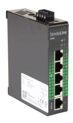
StrideLinx Basic industrial VPN router, wired Internet connectivity, (5) Ethernet Gigabit (RJ45) port(s), Android/iOS with mobile VPN, 12-24 VDC required.
