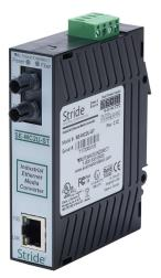
STRIDE industrial unmanaged Ethernet media converter, 2 ports, (1) Ethernet 10/100Base-T (RJ45) and (1) multi-mode ST 100FX fiber port(s), -10 to +60 deg C, plastic housing, IP40, 35mm DIN rail mount, hazardous location rated.
