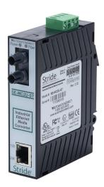
STRIDE industrial unmanaged Ethernet media converter, 2 ports, (1) Ethernet 10/100Base-T (RJ45) and (1) multi-mode ST 100FX fiber port(s), -10 to +60 deg C, plastic housing, IP40, 35mm DIN rail mount, hazardous location rated.
