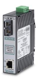
STRIDE industrial unmanaged Ethernet media converter, 2 ports, (1) Ethernet 10/100Base-T (RJ45) and (1) multi-mode SC 100FX fiber port(s), -10 to +60 deg C, plastic housing, IP40, 35mm DIN rail mount, hazardous location rated.
