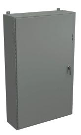
Wiegmann disconnect enclosure, NEMA 12/13, right flange, 60 x 37 x 12in (HxWxD), wall mount, carbon steel, ANSI 61 gray, powder coat finish, single-door, 3-point padlocking handle, purchase subpanel separately.
