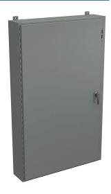
Wiegmann disconnect enclosure, NEMA 12/13, right flange,  $60 \times 37 \times 8$  in (HxWxD), wall mount, carbon steel, ANSI 61 gray, powder coat finish, single-door, 3-point padlocking handle, purchase subpanel separately.
