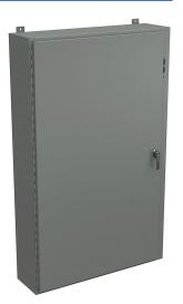
Wiegmann disconnect enclosure, NEMA 12/13, right flange, 60 x 37 x 10in (HxWxD), wall mount, carbon steel, ANSI 61 gray, powder coat finish, single-door, 3-point padlocking handle, purchase subpanel separately.
