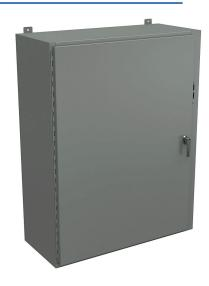
Wiegmann disconnect enclosure, NEMA 12/13, right flange, 48 x 37 x 16in (HxWxD), wall mount, carbon steel, ANSI 61 gray, powder coat finish, single-door, 3-point padlocking handle, purchase subpanel separately.
