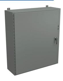
Wiegmann disconnect enclosure, NEMA 12/13, right flange, 42 x 37 x 12in (HxWxD), wall mount, carbon steel, ANSI 61 gray, powder coat finish, single-door, 3-point padlocking handle, purchase subpanel separately.
