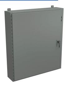
Wiegmann disconnect enclosure, NEMA 12/13, right flange, 42 x 37 x 8in (HxWxD), wall mount, carbon steel, ANSI 61 gray, powder coat finish, single-door, 3-point padlocking handle, purchase subpanel separately.
