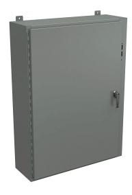
Wiegmann disconnect enclosure, NEMA 12/13, right flange, 42 x 31 x 10in (HxWxD), wall mount, carbon steel, ANSI 61 gray, powder coat finish, single-door, 3-point padlocking handle, purchase subpanel separately.
