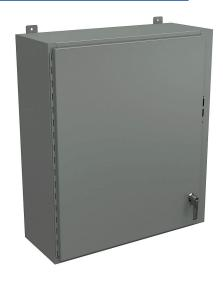
Wiegmann disconnect enclosure, NEMA 12/13, right flange, 36 x 31 x 12in (HxWxD), wall mount, carbon steel, ANSI 61 gray, powder coat finish, single-door, 2-point padlocking handle, purchase subpanel separately.
