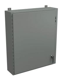
Wiegmann disconnect enclosure, NEMA 12/13, right flange, 36 x 31 x 8in (HxWxD), wall mount, carbon steel, ANSI 61 gray, powder coat finish, single-door, 2-point padlocking handle, purchase subpanel separately.
