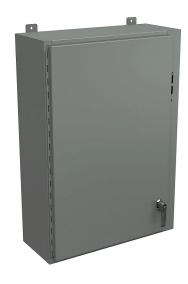
Wiegmann disconnect enclosure, NEMA 12/13, right flange, 36 x 25 x 10in (HxWxD), wall mount, carbon steel, ANSI 61 gray, powder coat finish, single-door, 2-point padlocking handle, purchase subpanel separately.
